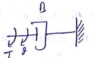
ideal rotational dash-pot with one end fixed.
