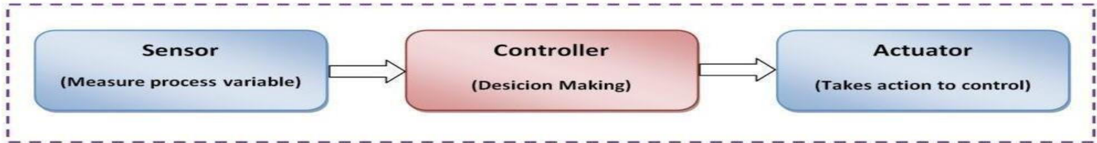
Figure- Sensor and actuator in a system
