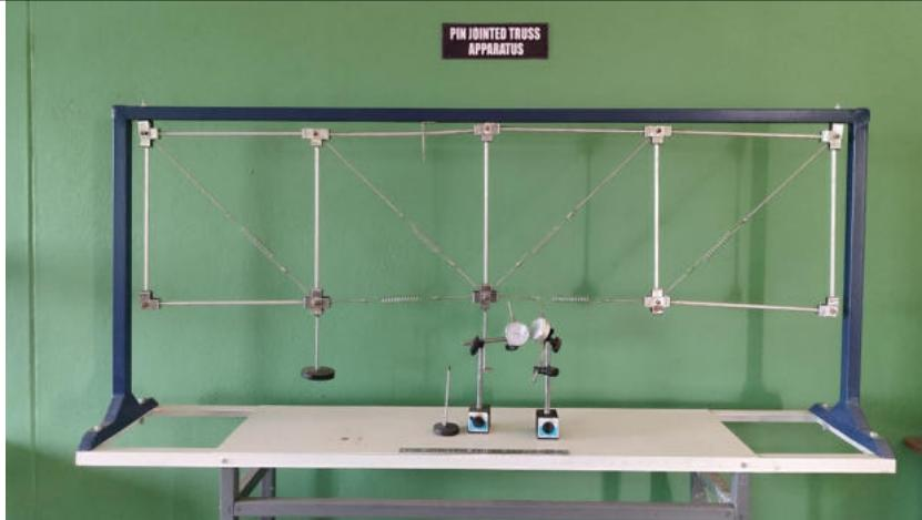
A photograph of a Pin Jointed Truss Apparatus. It consists of a blue rectangular frame with internal diagonal and horizontal members. Four vertical rods are attached to the top of the frame, each ending in a hanger. A central vertical rod supports a circular dial gauge. The apparatus is mounted on a white rectangular base with a metal frame. | Pin Jointed Truss Apparatus | <ul style="list-style-type: none"> <li>• Loads applied using hangers and slotted weights (range: 0–1 kg each).</li> </ul>
