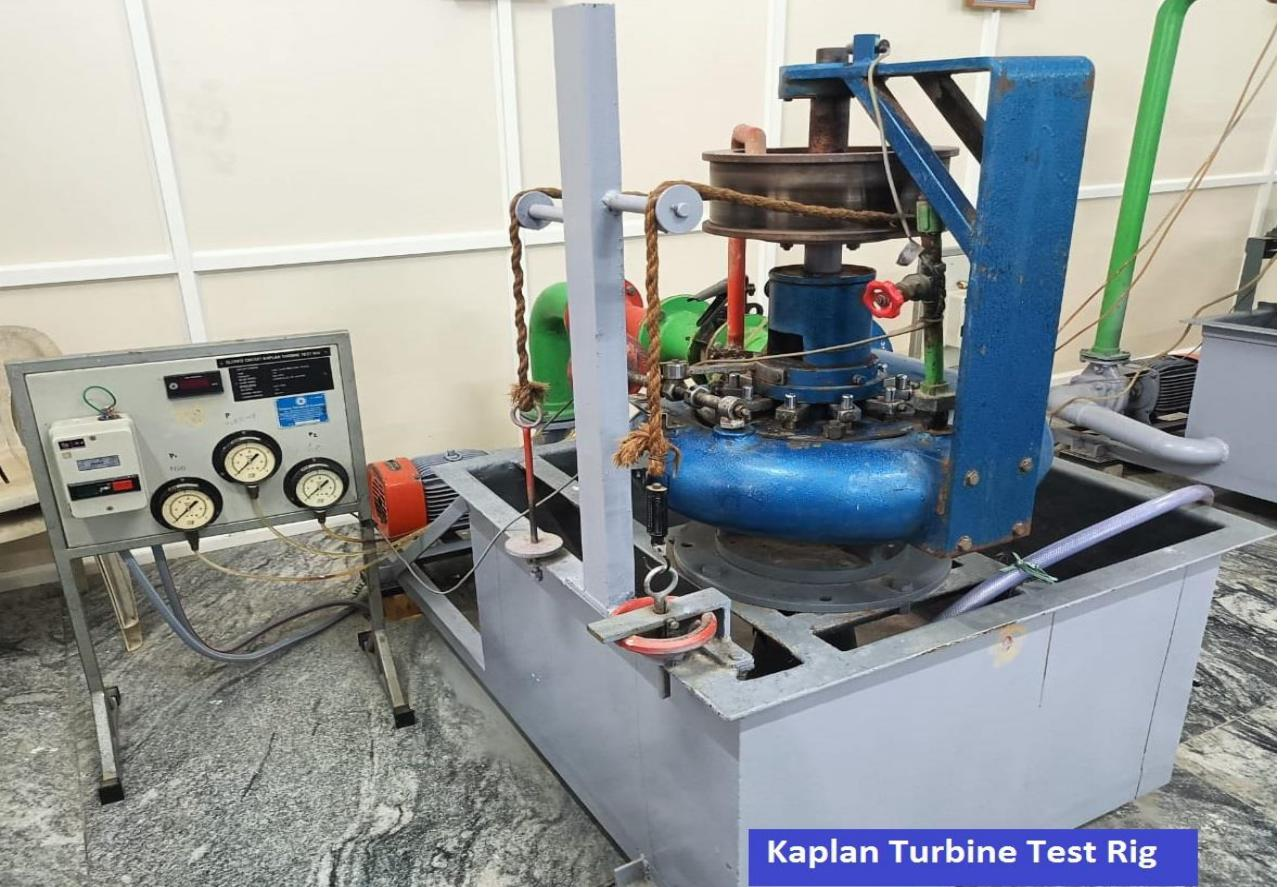
A photograph of a Kaplan Turbine Test Rig. The rig consists of a blue cylindrical turbine unit mounted on a grey metal frame. To the left, there is a control panel with a digital display and several analog pressure gauges. A red motor is connected to the turbine. Various pipes, hoses, and a green vertical pipe are visible, along with a blue support structure. A blue label at the bottom right of the rig reads "Kaplan Turbine Test Rig". |                                |
